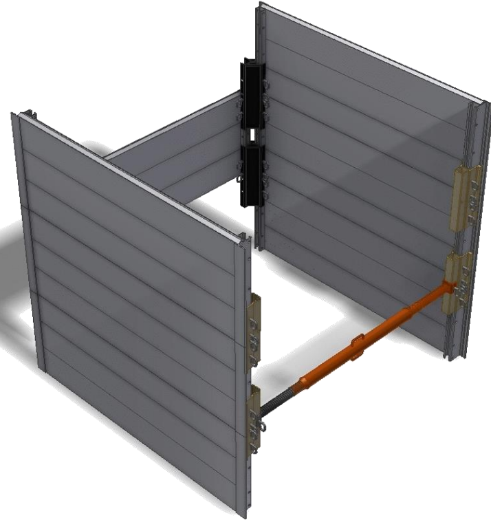
Step-10 With the panel connectors in place, install the appropriate LSS model strut Note that the each strut comes with one unpainted galvanized end and one painted. Make sure to match up ends when using Multiple struts. The paint code is an indication of direction the strut will adjust.
