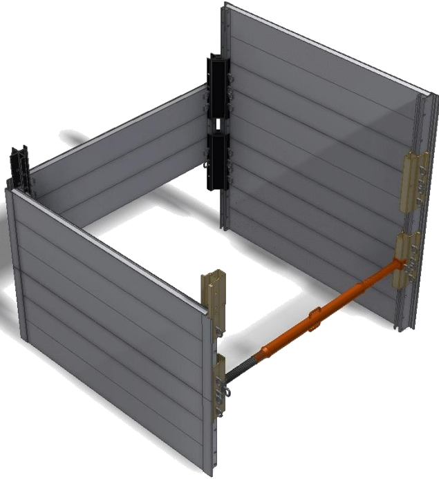
Step-9 On the south end, install 2 panel connectors (1 on each east and west panels.)
