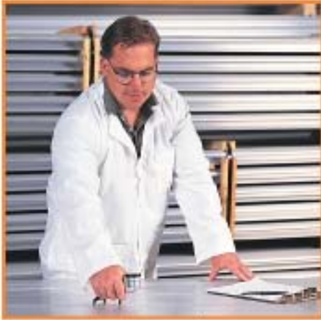
Incoming materials are routinely checked for hardness and acceptable surface finish.
